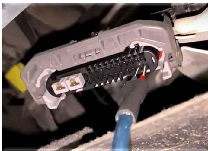
Connection to the CAN bus using the cable with needles
