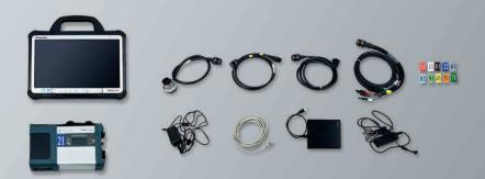
Workshop staff may use the XENTRY Connect with either the XENTRY Tab or a standard PC.
