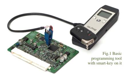
**TK-Prog** is advanced equipment set for electronic smart-key registration within Lexus and Toyota passenger cars (model year 2006-2014):
