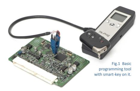
**TK-Prog** is advanced equipment set for electronic smart-key registration within Lexus and Toyota passenger cars:
