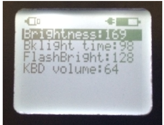
Pic.11 Settings menu with DC-power and USB connection indication.
