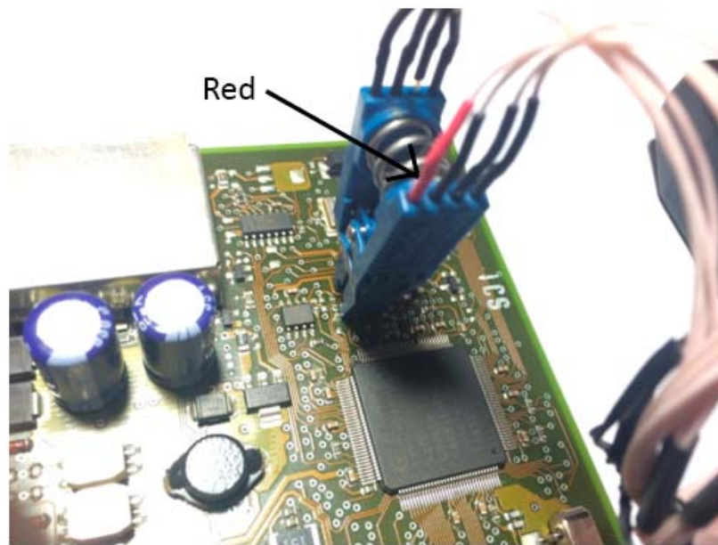
Pic.3 Connection with EEPROM chip on Kessy unit board.
