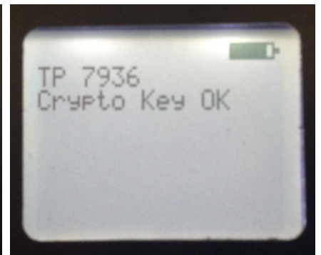
Pic.10 Message for key or chip that had been already registered in current Kessy unit.
